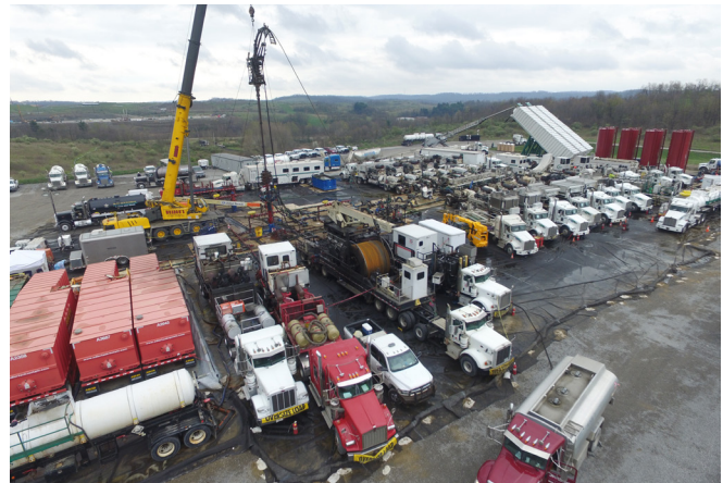
High Rate Annular Coiled Tubing Fracturing Operation. Calfrac Well Services Photo
